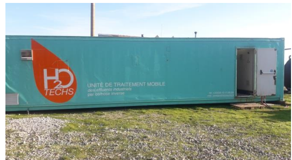
Figure 29. Station ENKI 4 120 m 3 /j en location
